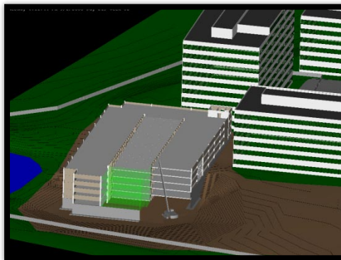
Figure 16 – Phase 1, Precast Sequence 6
